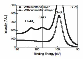
Figure shows the Si 2p peak at the interface for both sample with and without SiO<sub>2</sub>
