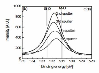
This O 1s peak position is in between Metal-O and Si-O for the sample with SiO<sub>2</sub> interfacial layer; indicating formation of silicates at the surface also at the interface
